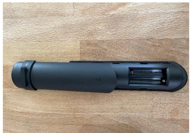
2. There is a clip that can be used to hook over a rail or frame. The batteries are located under the back cover.
