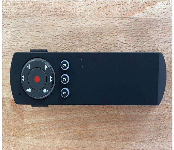
The Brick is the Control box which is connected to the motor using the cable via the larger 8 PIN connector on the Brick and Motor. The Wireless controller has a Red button for setting the controller to enable memory settings and control one motor or sync two motors together (see below). The left round icons control the head/back motions (up and down) and the right flat icons control the foot section (up and down). There are three memory buttons to memorize the adjustable settings.
